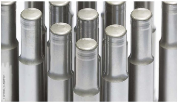
Milling punches from carbide: CCDia<sup>®</sup>CarbideSpeed<sup>®</sup> ensures excellent surface finishes.
