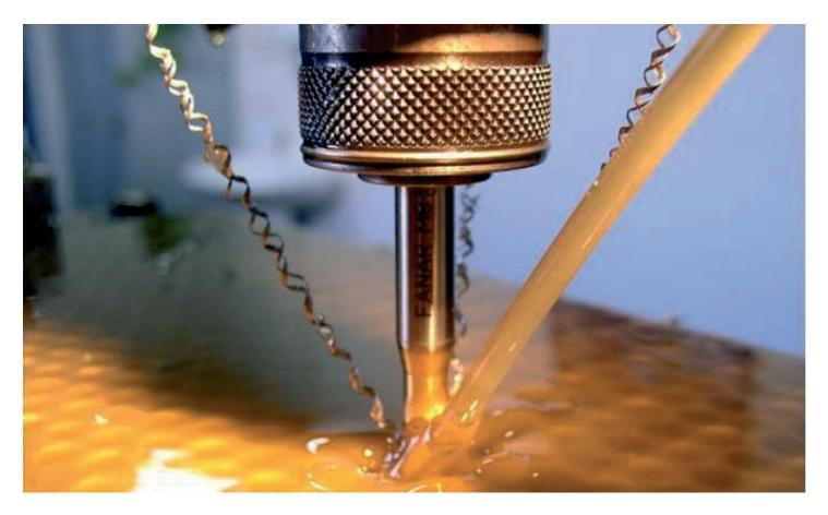
The threading is particularly important as the last machining step because a flaw here can ruin all the previous work. Therefore, a stable, reliable process is crucial. "The most important element for this is highquality tap drills with a coating that has low friction and good tribological properties," said Dariusz Ptaszkiewicz, Chief Technology Officer (CTO) at FANAR. "The smooth, droplet-free sputter coatings from CemeCon are therefore our first choice for our tap drills."
