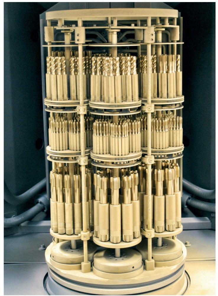
FANAR and CemeCon worked closely together to develop a premium coating that was designed precisely to the tap drill requirements. The prerequisite was higher wear resistance and longer tool life as compared
