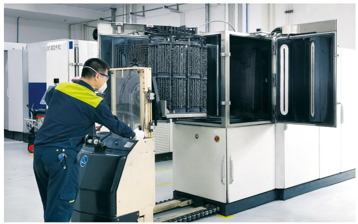
Huarui has been using sputter systems for coatings for a long time. To increase the performance of their inserts even further, Huarui is now investing in a CC800<sup>®</sup> HiPIMS.
