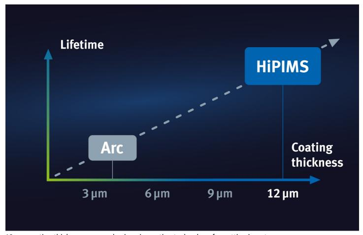
12 μm coating thickness – a new horizon in coating technology for cutting inserts.
