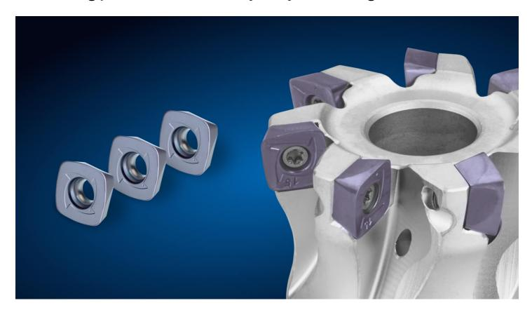
In heavy-duty machining of ferrous materials, tool life is directly proportional to coating thickness. With FerroCon®Quadro, CemeCon achieves coating thicknesses of up to 12  $\mu$ m on cutting inserts, making it the thickest PVD-based coating on the market. Compared to the CVD process, HiPIMS technology offers advantages such as smoother and tougher coatings, greater flexibility, more stable process control at lower temperatures and the possibility of targeted management of residual stresses.
