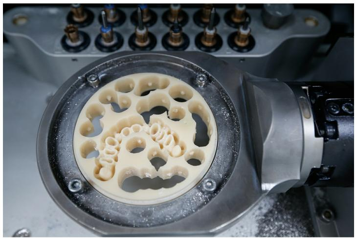
Known as the green compact (before the ceramics are fired), zirconium oxide is highly abrasive and porous at the same time. The wear resistance of cutting tools presents challenges to processing.
