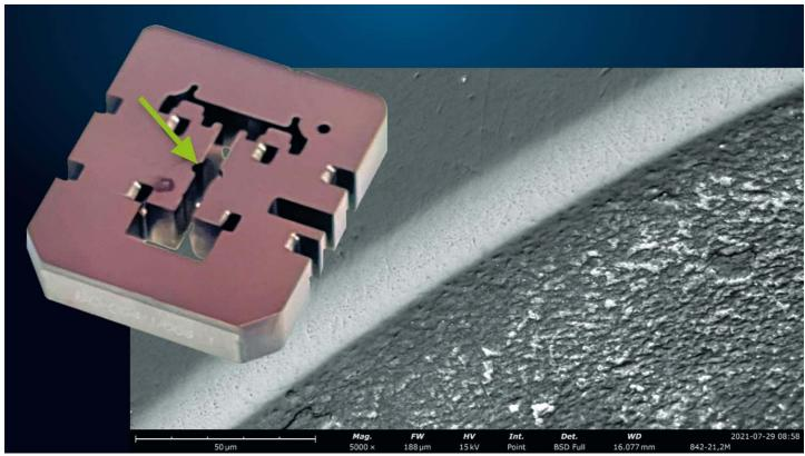
Even after 21.2 million strokes, the cutting die coated with InoxaCon® still has an unchanged edge. (Photos: Stepper)
