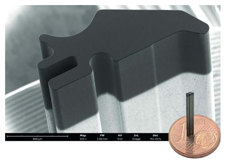
HiPIMS technology allows the filigree geometry of the cutting punch to be optimally coated. (Photos: Stepper)
