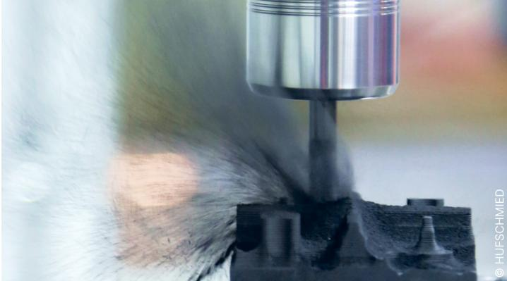
Diamond coatings from CemeCon offer the ideal solution for milling graphite electrodes © HUFSCHMIED
