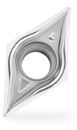
Extremely smooth and with layer thicknesses of only 2  $\mu$ m, AluCon® is highly effective in preventing built-up edges from forming in the first place
