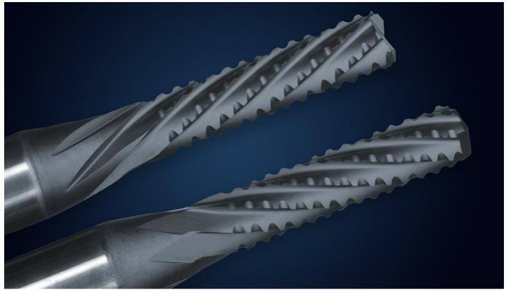
The new micro-milling cutters "HPTec Composite Tool Action" (top: downcut geometry; bottom: upcut geometry) have been precisely adapted to the machining of fiber composite plastics. An important component is the diamond coating based on CCDia®AeroSpeed®.
