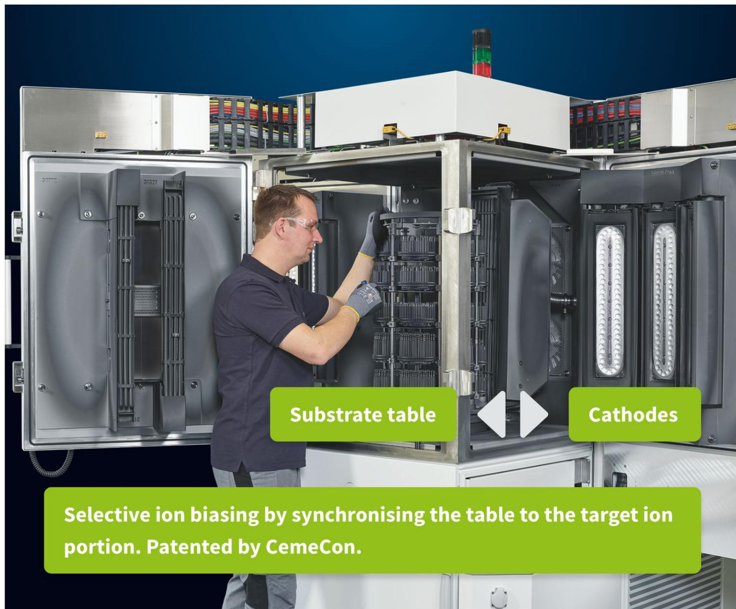
Synchronization of the HiPIMS pulses of the cathodes with the substrate table
