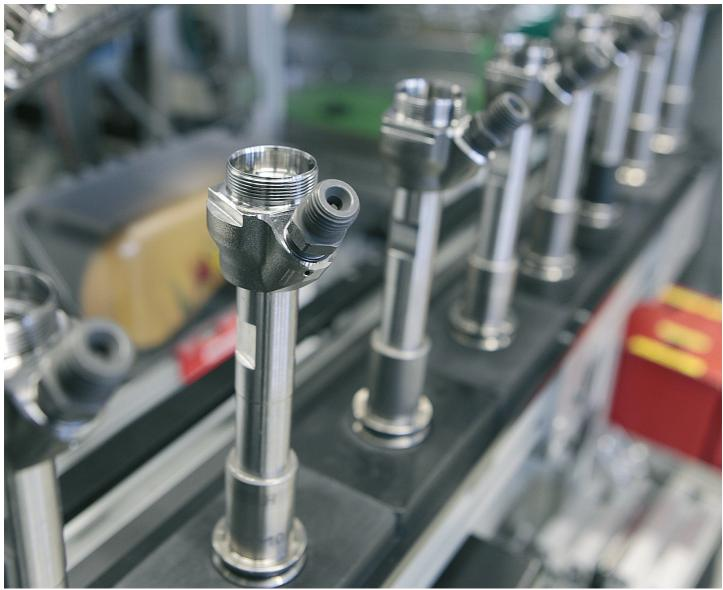
With HiPIMS Bosch was able to achieve higher component quality with increased process reliability in the production of common rail injectors.
