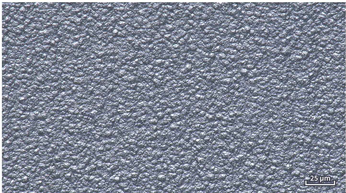
The diamond coating adapted for the new premium tool—shown here magnified 1,000 times—ensures a
