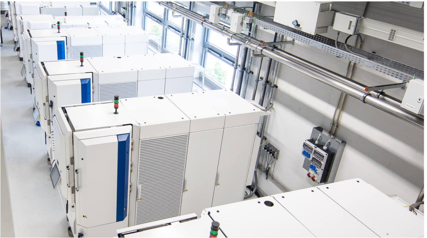
Horn has expanded its in-house coating centre with seven new CC800<sup>®</sup>-HiPIMS systems.
