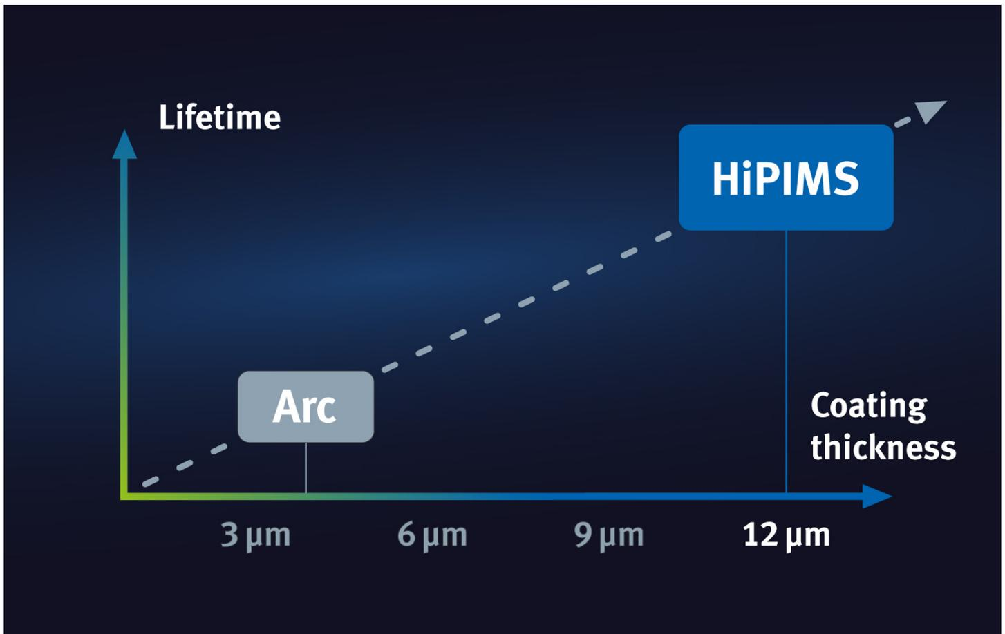
12  $\mu\text{m}$  coating thickness – a new horizon in coating technology for cutting inserts.
