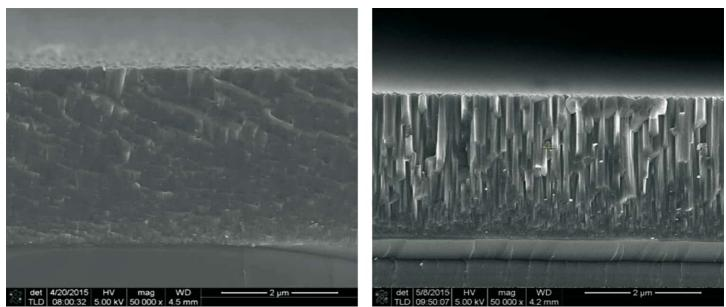
The comparison of the SEM images makes it very clear: thanks to the production in the HiPIMS process, AluCon<sup>®</sup> (right) has a much finer structure than AluSpeed<sup>®</sup> (left) and thus improved coating properties
