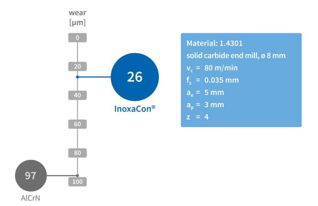
A practical example in comparison with AlCrN underscores the efficiency of the HiPIMS coating material.
