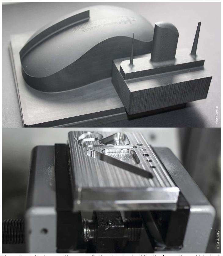
Diamond-coated tools are used in many applications: in tool and mold making for graphite machining (top) or aluminum (bottom). Customized solutions bring clear competitive advantages here. (Photos: HUFSCHMIED)
