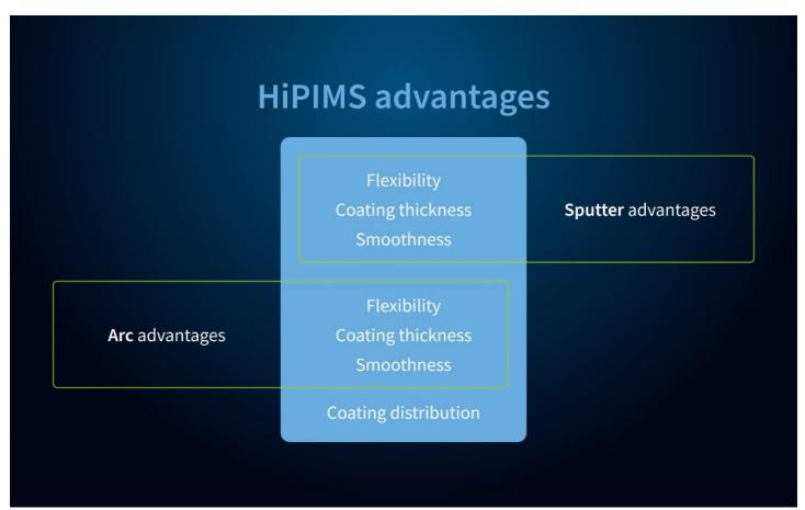
HiPIMS (High Power Impulse Magnetron Sputtering) is the further development of sputtering technology and combines the advantages of all current coating technologies and processes available on the market.
