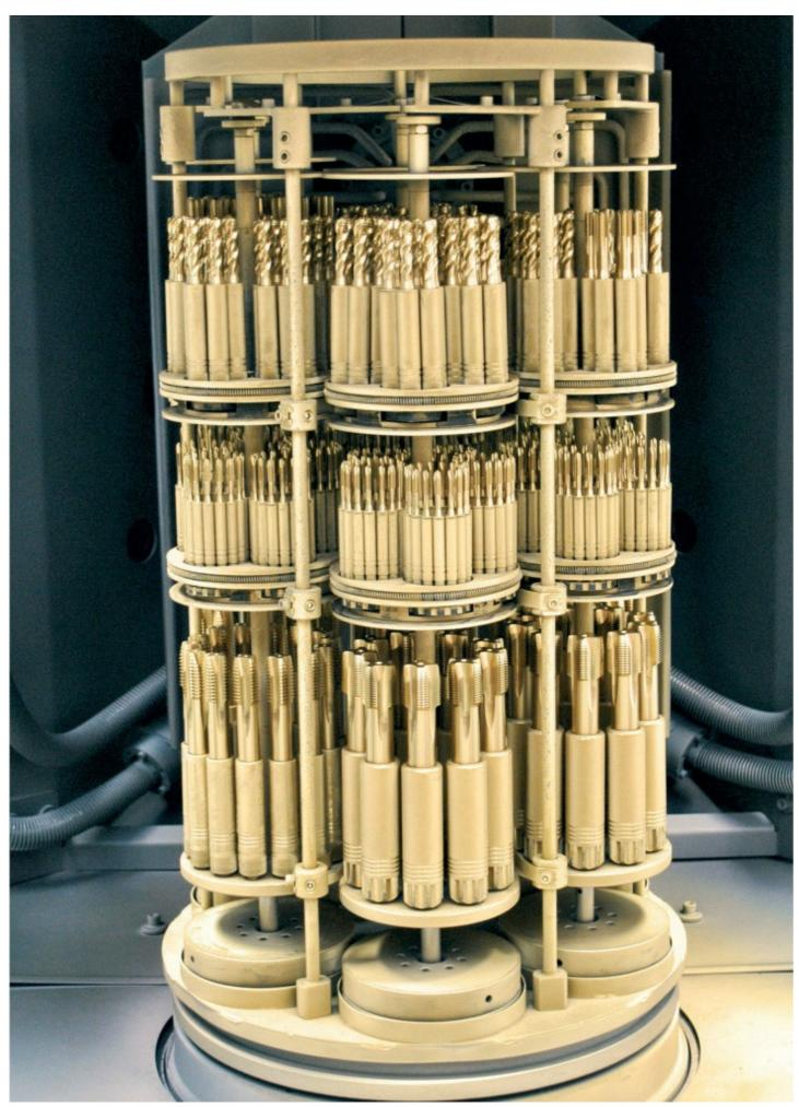
FANAR and CemeCon worked closely together to develop a premium coating that was designed precisely to the tap drill requirements. The prerequisite was higher wear resistance and longer tool life as compared
