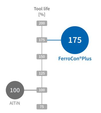
Material: 1.0552 ( $R_m = 520 \text{ N/mm}^2$ ) Solid carbide drill, ø 15.1 mm  $v_c = 180 \text{ m/min}$ f = 0.36 mm
