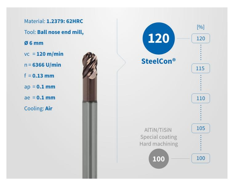
Since no droplets can form thanks to the HiPIMS process, SteelCon® is extremely smooth. This means that nothing stands in the way of optimum chip and heat removal. The tool can dissipate the heat in the chips, and process stability increases. Excellent surface qualities are achieved, so that the user can often save subsequent work – in some cases even the polishing of their workpieces.
