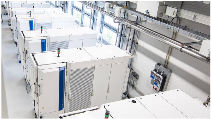
Horn has expanded its in-house coating centre with seven new CC800°-HiPIMS systems.
