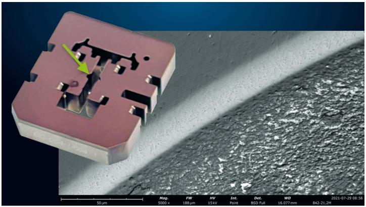
Even after 21.2 million strokes, the cutting die coated with InoxaCon<sup>®</sup> still has an unchanged edge. (Photos: Stepper)
