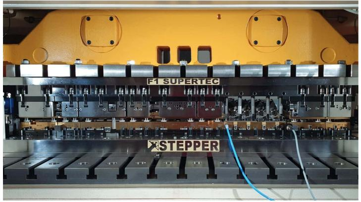
Modular progressive dies from Stepper can incorporate over 1,000 PVD-coated moving active parts, such as cutting punches, cutting, bending and embossing inserts. Excessive wear on any one of these active parts affects product quality. With HiPIMS technology, Stepper can significantly extend required maintenance intervals (typically to well over 10 million punch strokes without maintenance intervention).
