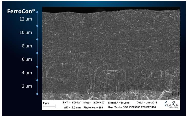
FerroCon<sup>®</sup>Quadro with 12 μm coating thickness – the advantage for roughing operations
