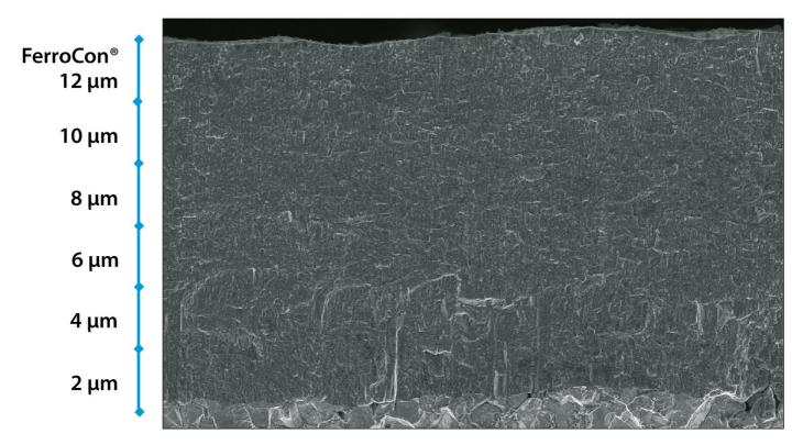
FerroCon®Quadro with a coating thickness of up to 12  $\mu$ m – the HiPIMS technology from CemeCon makes it possible.
