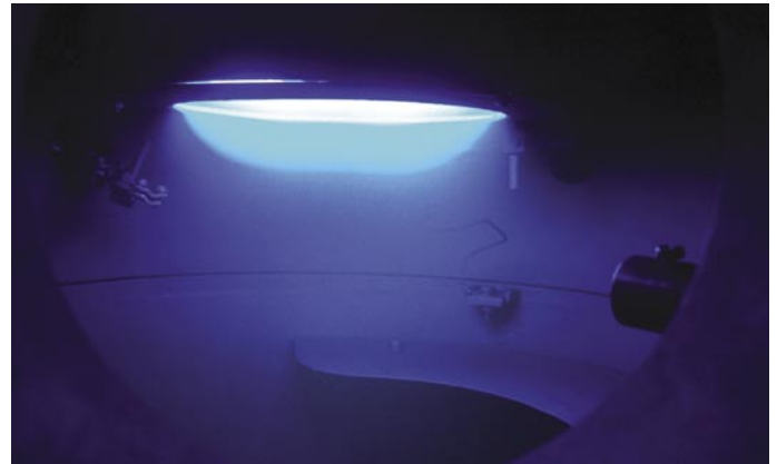
HiPIMS: with high pulses to adhesive coatings.
