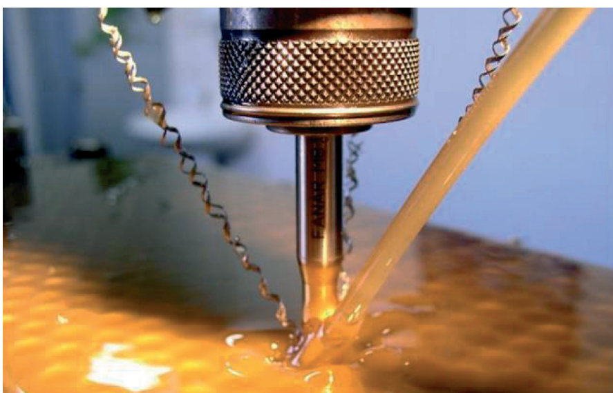
Fanar TN coating – a droplet-free sputter layer – offers users new possibilities in tapping. (Photo: FANAR)
