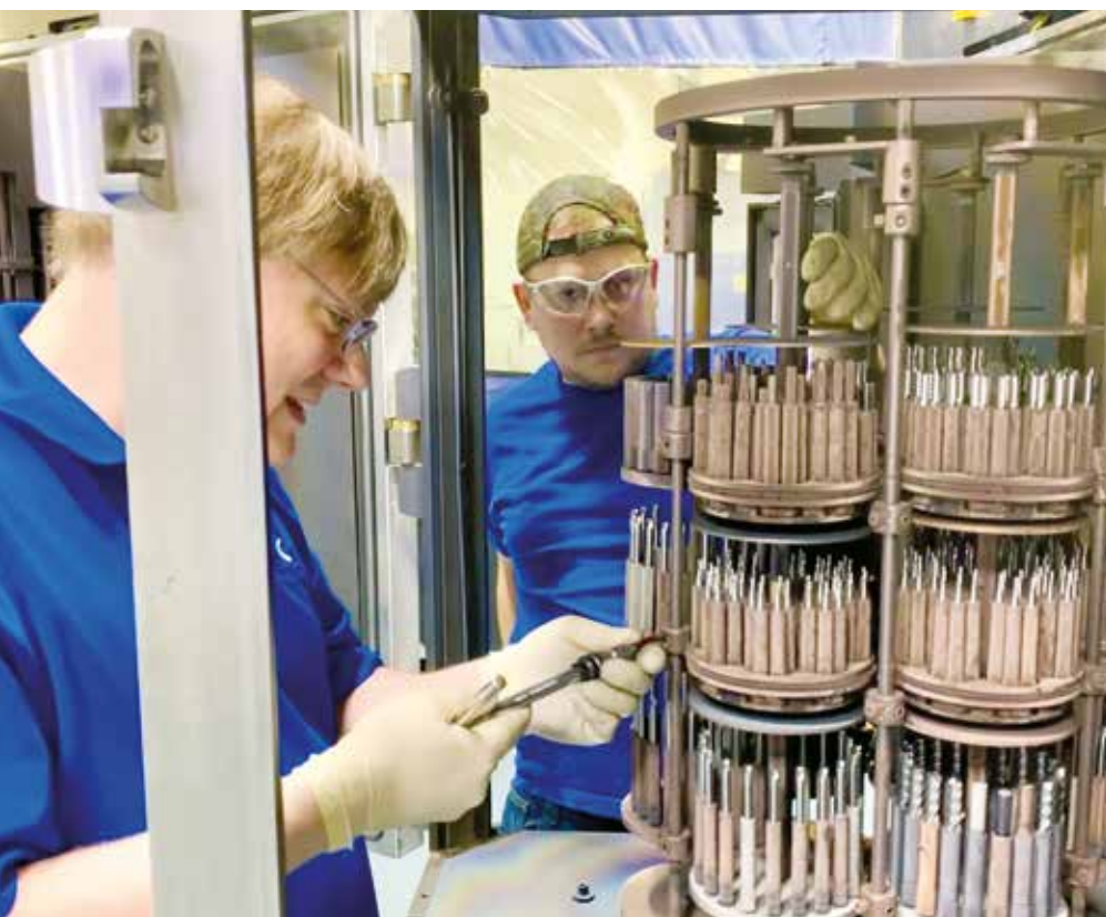
Handling is really simple: Scott Para (left) and Brandon Wilkins load the CC800® HiPIMS coating chamber.
