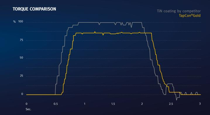
A stable low torque is enormously important for precise and efficient thread production. The newly developed HiPIMS coating material TapCon®Gold was tailored specifically to these requirements and is the ideal coating base for HSS taps and thread formers.
