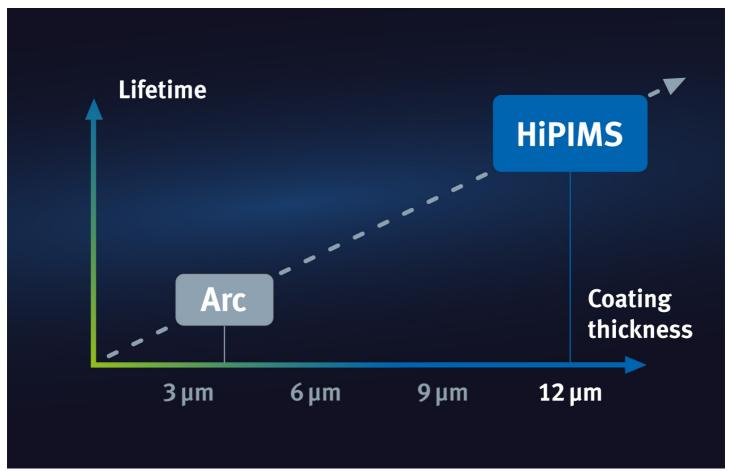
12  $\mu$ m coating thickness – a new horizon in coating technology for cutting inserts.
