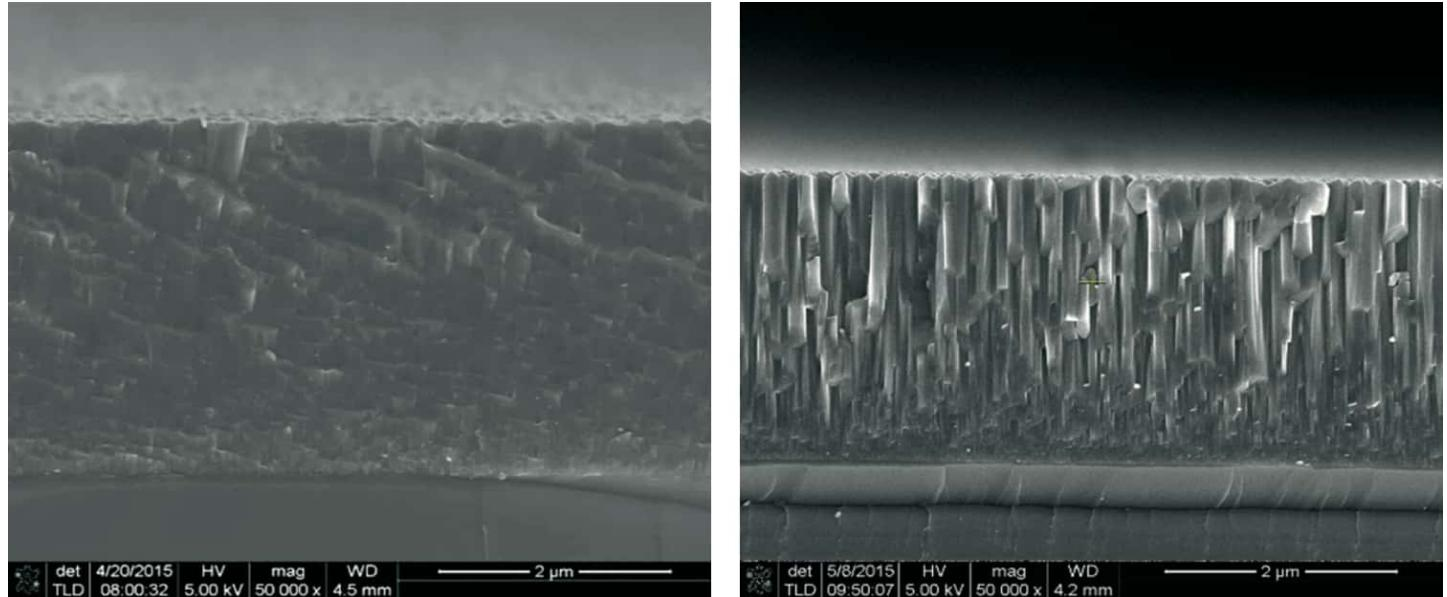
The comparison of the SEM images makes it very clear: thanks to the production in the HiPIMS process, AluCon® (right) has a much finer structure than AluSpeed® (left) and thus improved coating properties
