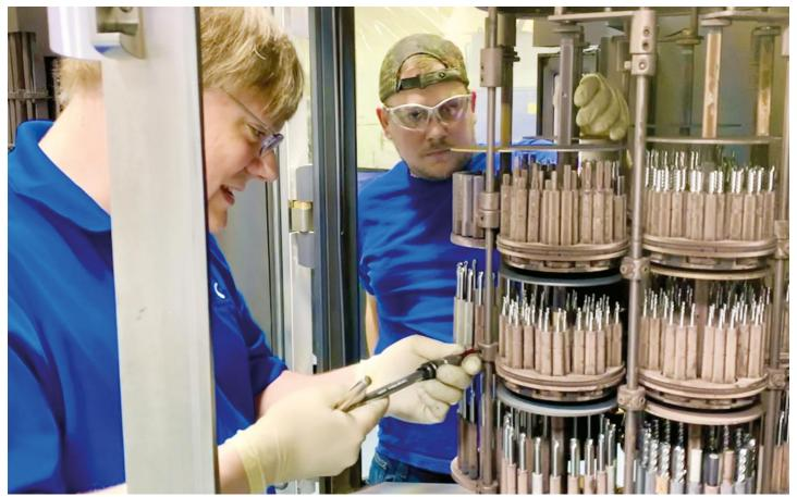
Handling is really simple: Scott Para (left) and Brandon Wilkins load the CC800® HiPIMS coating chamber.
