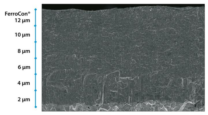
FerroCon<sup>®</sup>Quadro with a coating thickness of up to 12  $\mu m$  – the HiPIMS technology from CemeCon makes it possible.
