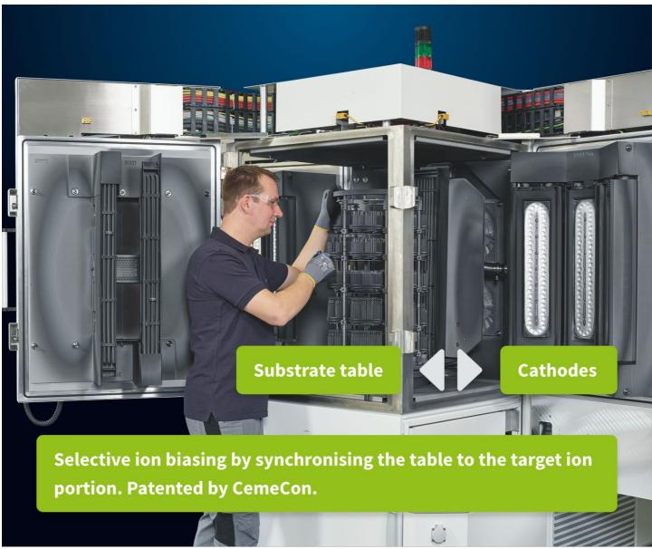
Synchronization of the HiPIMS pulses of the cathodes with the substrate table
