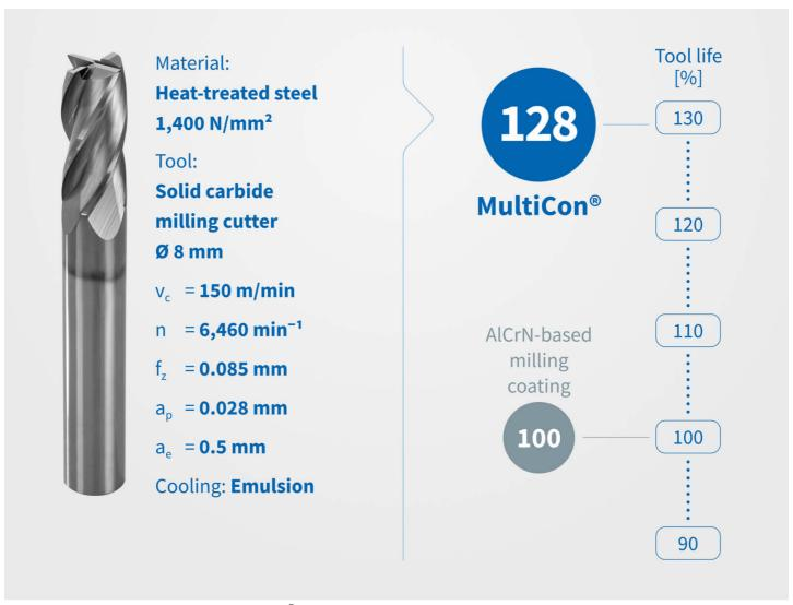
Practical examples show how MultiCon<sup>®</sup> increases productivity. When milling heat-treated steel (1,400 N/mm<sup>2</sup>), the tool life was increased by almost 30 percent compared to an AlCrN coating deposited using arc technology.
